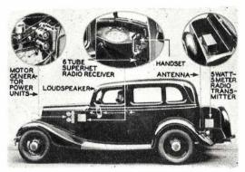
The above illustrates the manner in which the two-way radio-telephone equipment operates. The antenna projects above the back of the car, with the transmitter in the trunk.
