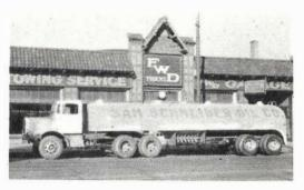
As long as the average freight car, this streamlined gasoline truck is used to make deliveries in sparsely settled areas. The 18-ton load is distributed evenly over each of the 18 wheels.
