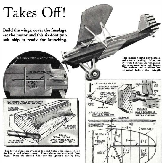
for those who prefer a steady flying somewhat slower job to a fast ship the larger span will commend itself. The centersection may also be increased to as much as a 12-inch span but in this event minor changes in the placing of the wing strut fittings will be necessary to avoid too wide a splay on the interplane struts.
