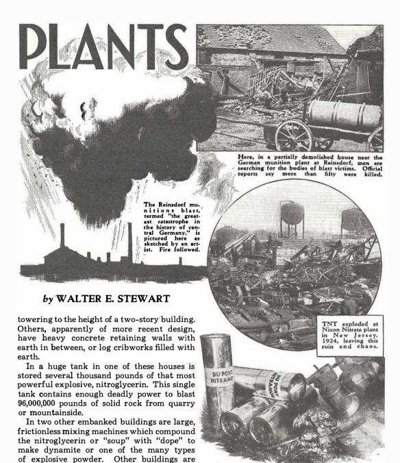
This new explosive, known as Nitramon, is immune to flames, and can be detonated only by a large charge of dynamite. Large supplies of Nitramon can be stored in safety, where ordinary stick dynamite or TNT would prove too hazardous.
