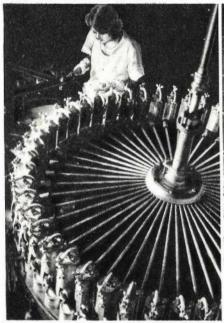
Above—Impregnating splints with boric acid solution to prevent afterglow when match is struck.
