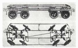
The double trucked trailer shown above eliminates side sway through an arrangement of tie rods and connecting rod operating on independently mounted wheels as shown below.
