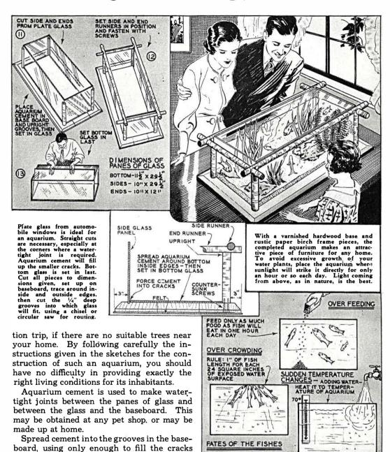
when the glass is set in. Now assemble the aquarium piece by piece, applying cement to each joint and to the insides of the corner posts. Block up the glass from the inside to
