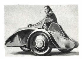
High speeds without sacrifice of comfort are possible in the streamlined motorcycle side car, shown above. The long slanting windshield provides ample protection from wind.
