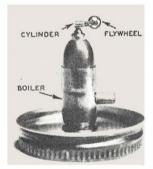
A .45 caliber shell provides the boiler for this tiny steam engine weighing only 1/170th of an ounce. It can make 15,000 r.p.m. on the steam created by a match.
