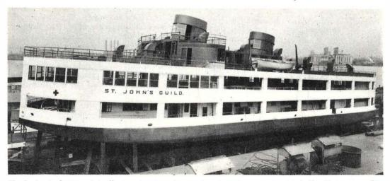
The St. John's Guild hospital ship, the safest boat afloat, is shown here about to be launched in New York harbor. The boat, built for the benefit of the poor children, is entirely fireproof, and has 25 watertight compartments to prevent sinking.
