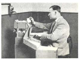
This robot letter sorter is operated by a keyboard on which the principal cities are designated by number. It is only necessary to press the required button and the letter is pouched.
