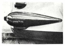
Projecting slightly from the buffer chamber of a French rail-car, this pneumatic tire adds to the streamlining of the novel car, while serving as both the bumper and the spare tire.
