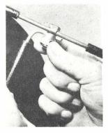
The jaws of this one-piece wire connector lock tightly together, insuring a non-breakable, positive contact that will not jar loose.
