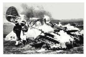
Not until the blazing airplane in which he was testing an asbestos suit was almost reduced to ashes did this inventor, shown at right, leave the cockpit. He was unharmed by heat.
