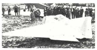
Already winning admiration in aviation circles is this "Flying Fish," the product of a French aviator. The outstanding features of this tailless plane are its exceptional stability in rough air and its ease of handling.
