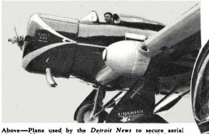
Above—Plane used by the Detroit News to secure aerial photos. Note the bullet-shaped compartment which houses the wing camera. Pilot controls camera from the cockpit.
