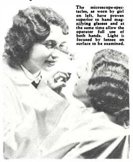
ADJUSTABLE lenses mounted on spectacle frames have been developed in Germany to replace low powered hand microscopes for use by doctors, laboratory workers, beauticians and others who require both hands for close work.
