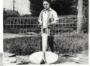
Skeleton construction of all wings is plainly visible in this photograph. Lower wings are shown without aluminum ends.
