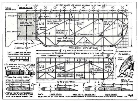
Complete wing construction is shown above. Center section is held to the fuselage with N struts shown in Fig. 1, Part I. which appeared in the August issue.
