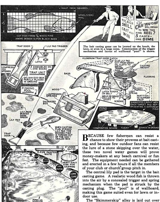
The "Skimmerskip" alley is laid out over calm water, with posts arranged as shown for markers. Prizes go to those who succeed in skipping a stone through the arch at the opposite end. As flat stones are scarce in most localities, heavy galvanized metal discs are used. These can be recovered with a long-handled rake.
