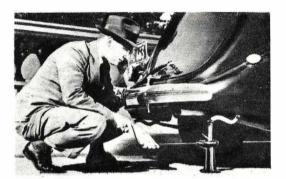
This extension bolted to the chassis side members at both front and rear provides an accessible jack rest on streamlined cars. Tire changing is much simplified by this improvement.
