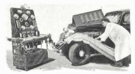
This motor analyzer is shown registering the efficiency of the generator on the car being tested. It detects any flaw in the ignition system, and also checks motor performance.
