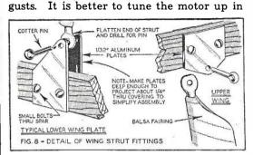
Cut the plates from aluminum and fasten to the spar as shown. Struts are faired in same manner as landing gear in Part I.
